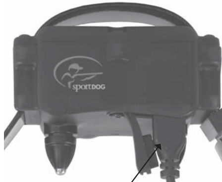
CHARGER CONNECTOR PLACED IN COLLAR RECEIVER CHARGING JACK
