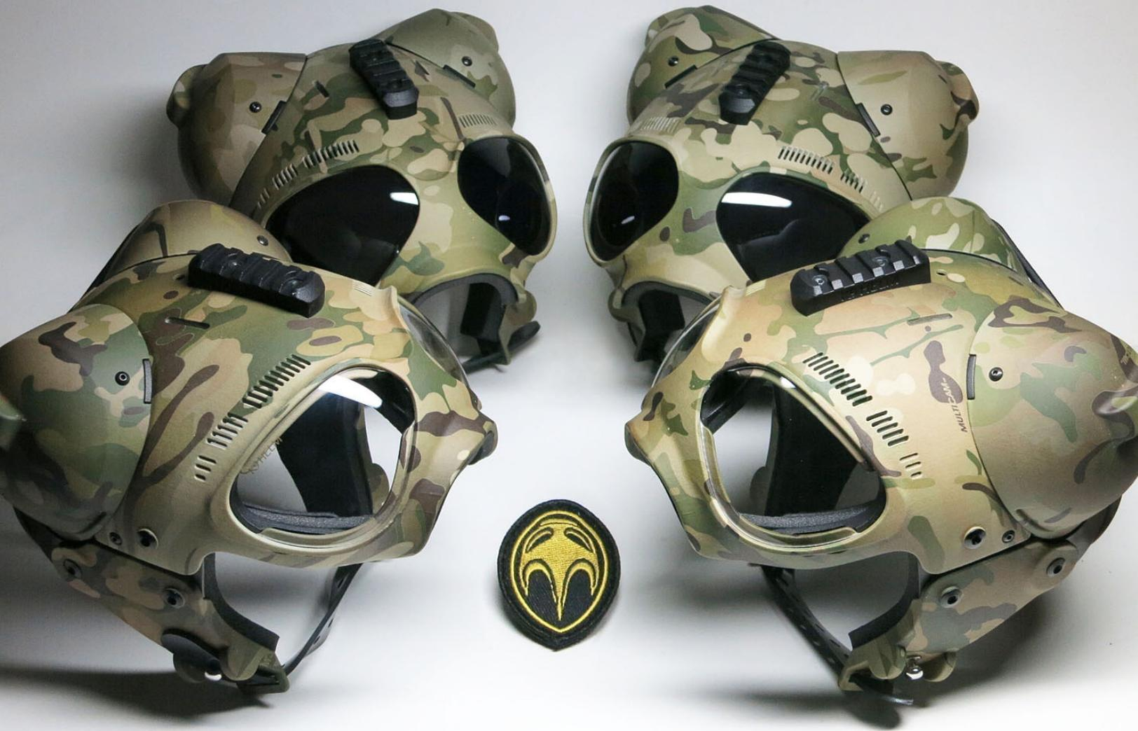
Nylon helmet shells are prepped with an epoxy primer and color coat. Then, the multicam pattern is applied using a hydro-dipping process. Finally, the parts are sprayed with a matte urethane clear coat. The vendor offering this service has an average lead time of 3-4 weeks.
